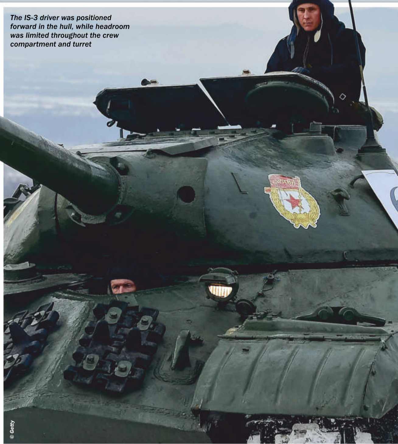
The cramped crew compartment and flattened turret of the IS-3 restricted the operation of the 122mm D25-T main weapon
